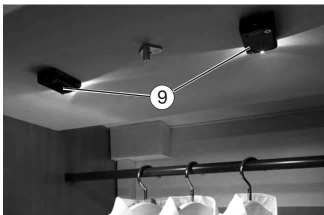
The clothes cupboard light ⑨ is switched on and off by opening the doors of the cupboard (integrated contact switch - cannot be switched on the control panel). The LED light is battery-operated. Before initial operation, pull off the foil that prevents battery contact.
