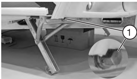
Hexagon head for front rotating stanchions in the ONTOUR/Landhaus models
