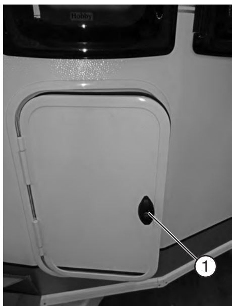
Door of the gas-bottle container
