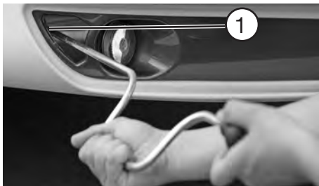
Hexagon head for front rotating stanchions in the De Luxe (Edition)/Excellent/Prestige/Premium models
