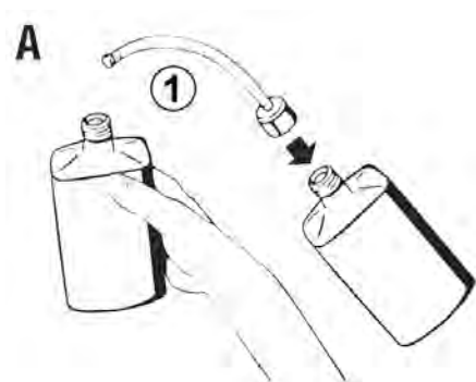
Open the fill hose on the bottle
