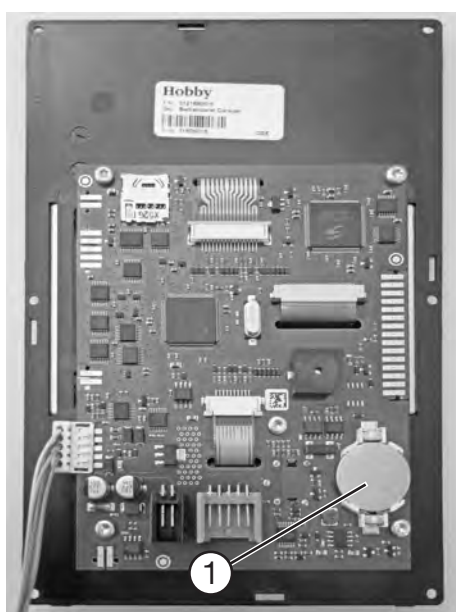
Circuit board (reverse side) of TFT display
