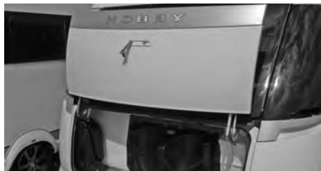
Opening the gas bottle container
