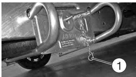
Thread locker on the spare tyre mount
