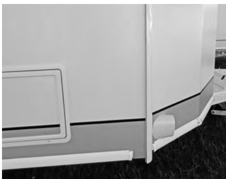
Outer tent guide rail with insertion for keder from below
