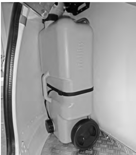
Waste water tank in the gas bottle container
