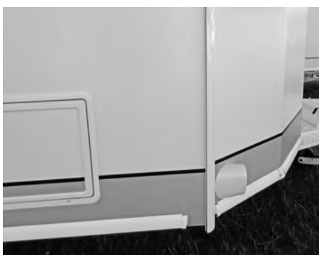
Outer tent guide rail with insertion for keder from below
