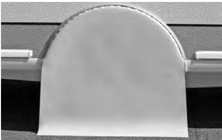
Wheel cover with integrated keder strip for mudguard
