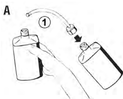
Open the fill hose on the bottle
