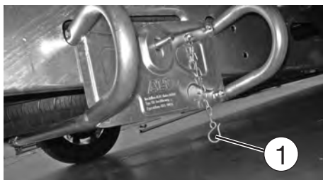
Thread locker on the spare tyre mount
