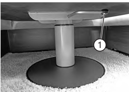
Lever ① to lower the table
