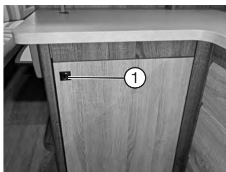
The carousel is safeguarded by means of a pushlock
