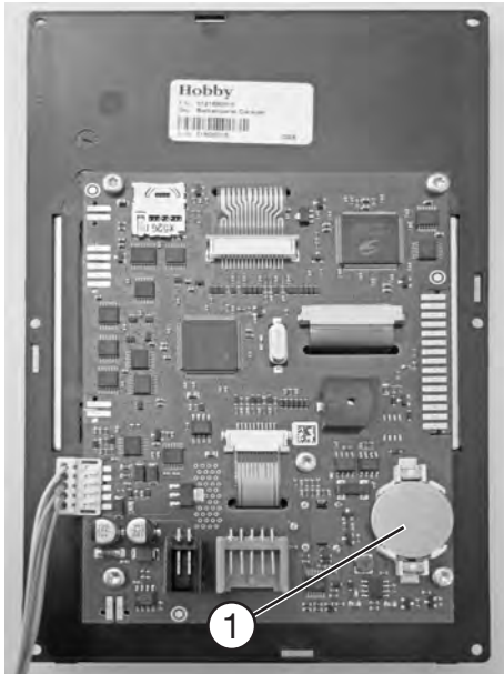
Circuit board (reverse side) of TFT display
