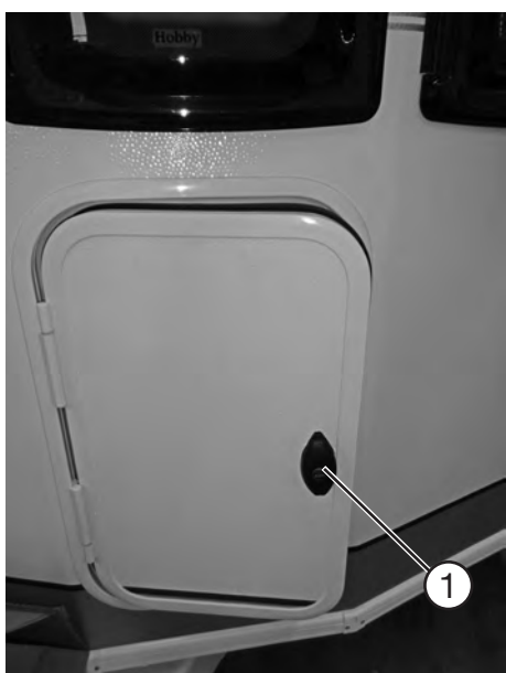
Door of the gas-bottle container
