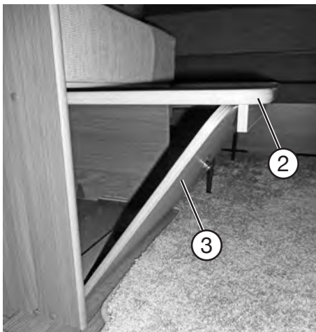
Widening the seating bench
