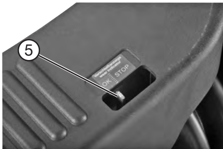
Wear indicator for the friction pads
