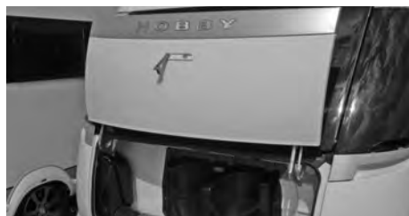
Opening the gas bottle container
