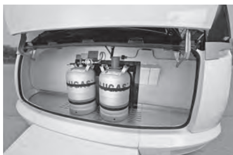
Positioning the gas bottle in the gas box
