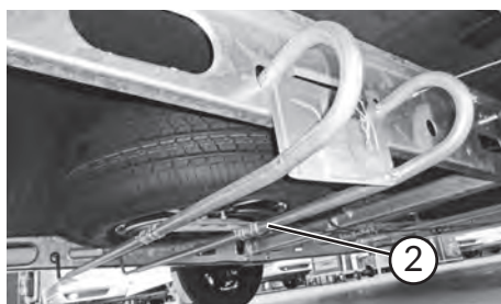
Spare wheel holder in chassis beam
