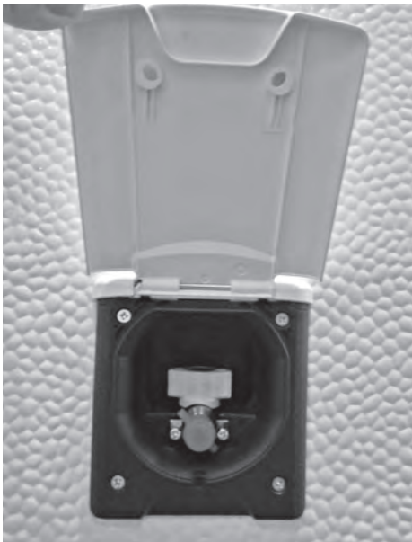
External gas socket
