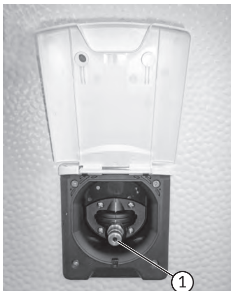
City water supply connection
