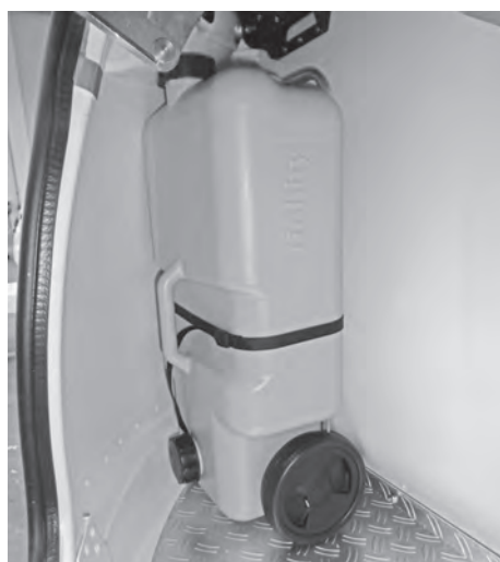
Waste water tank in the gas box
