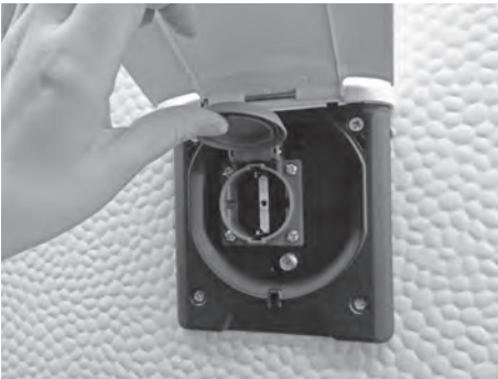
External socket and antenna terminal in the awning.
