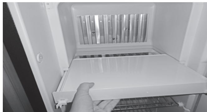
Removing the base of the freezer
