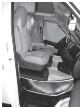
Footwell insulation in driver's cab
