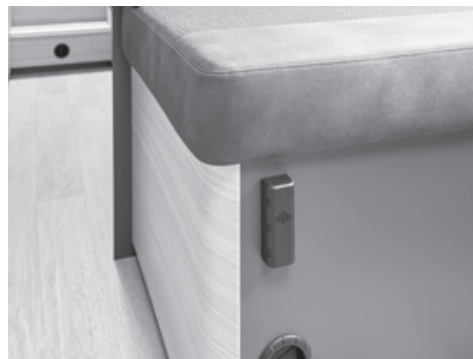
Gas warning system
