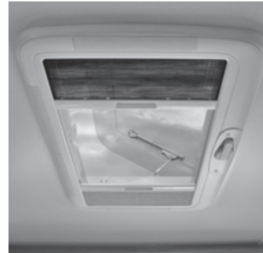
Large roof light
