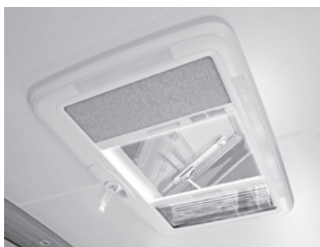
Large roof light
