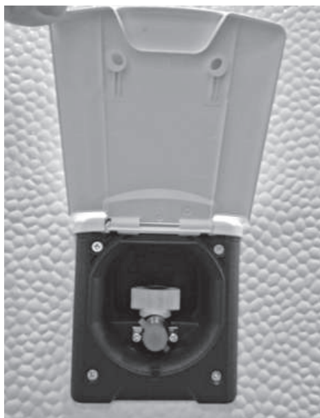
External gas socket
