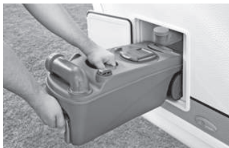
Emptying the waste tank (cassette)
