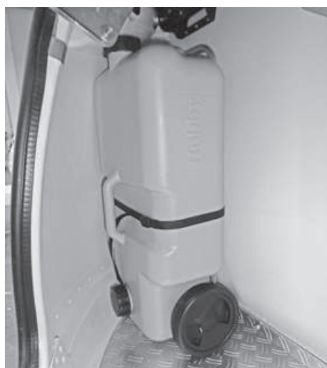
Waste water tank in the gas box
