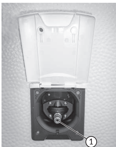
City water supply connection
