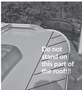
Curved edges of roof
