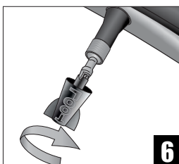
Screwing the valve core tight
