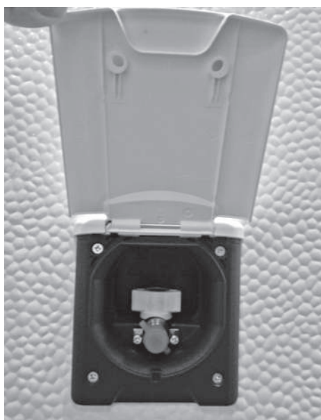
External gas socket
