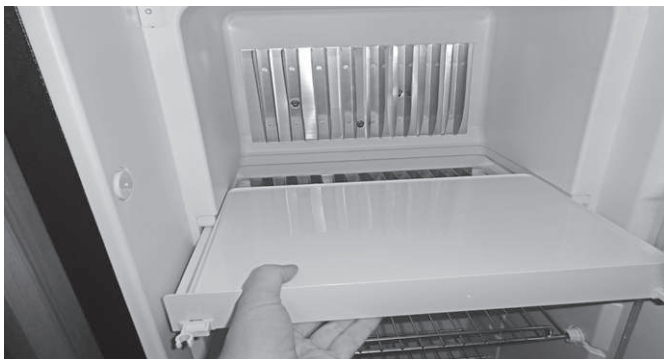
Removing the base of the freezer
