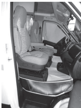
Footwell insulation in driver's cab
