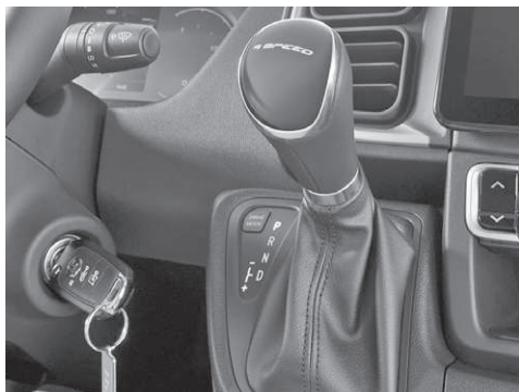
Selector lever on the automatic transmission
