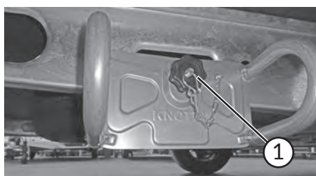
Threaded lock nut on the spare tyre mount
