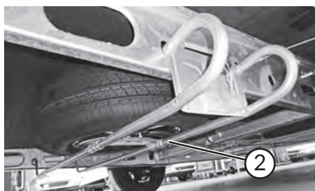
Spare wheel holder in chassis beam
