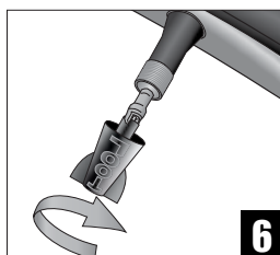
Screwing the valve core tight
