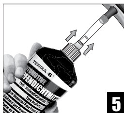
Pushing the filler hose onto the tyre valve
