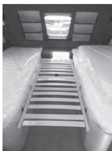
Hooking the slatted frame into place
