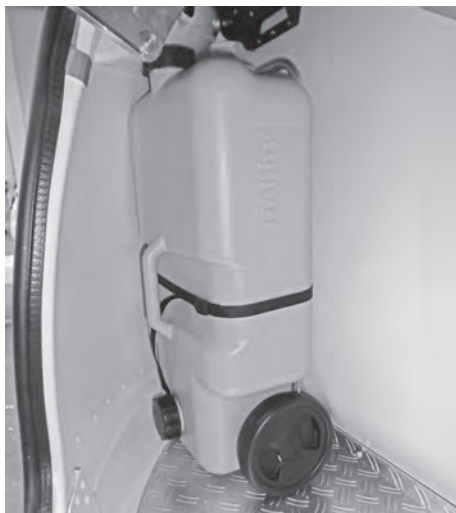
Waste water tank in the gas box
