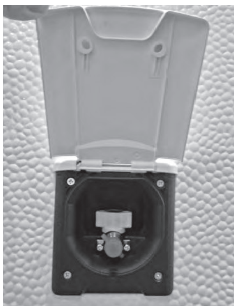
External gas socket
