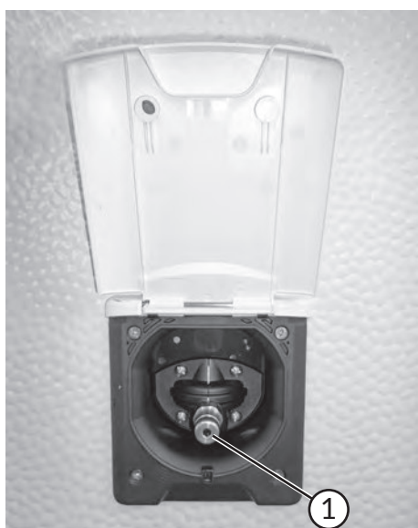
City water supply connection
