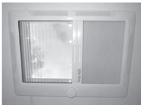
Large roof light
