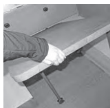
Hooking the table top into place
