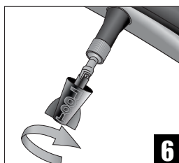
Screwing the valve core tight
