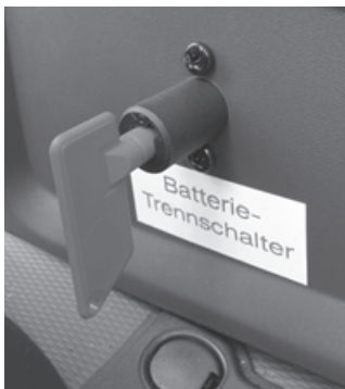
Battery circuit breaker
