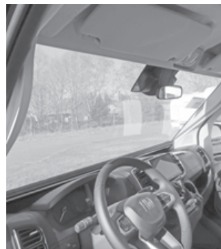
Blackout system for the wind-screen open
