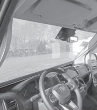
Blackout system for the wind- screen open
