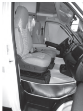
Footwell insulation in driver's cab
