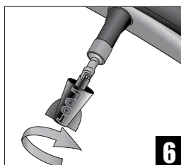
Screwing the valve core tight
