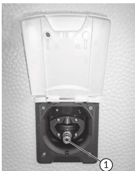
City water supply connection
