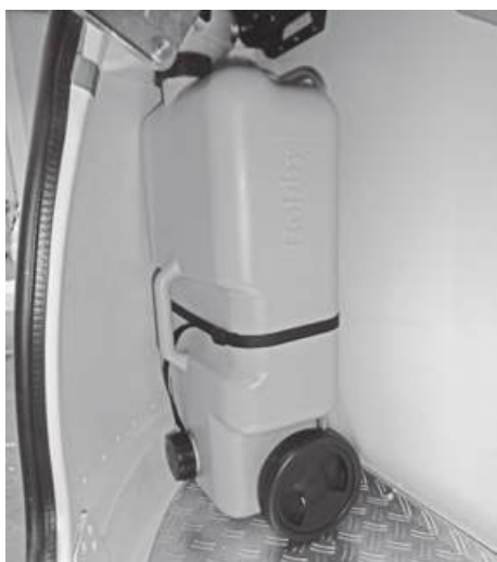
Waste water tank in the gas box
