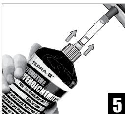
5 Pushing the filler hose onto the tyre valve
