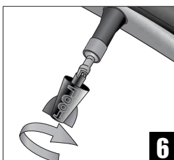
6 Screwing the valve core tight
