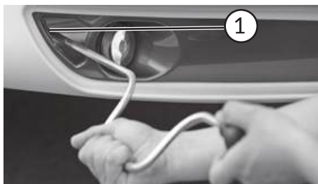
Hexagon head for heavy-duty supports in the front
