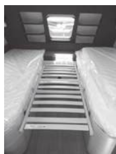
Hooking the slatted frame into place
